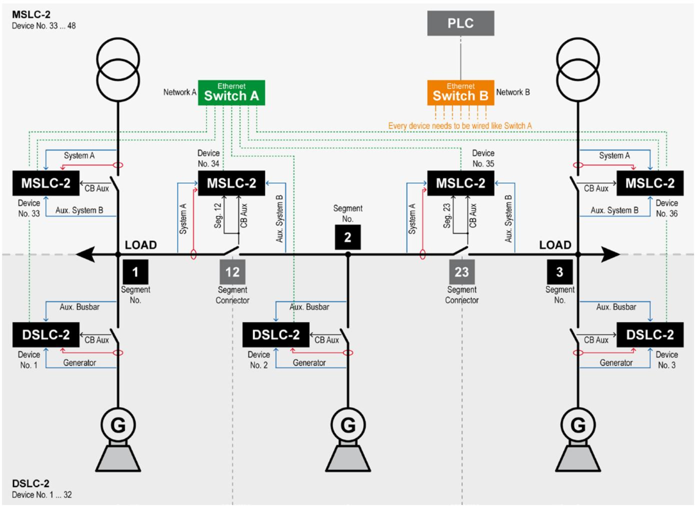
Configuration of a typical application using DSCLC-2™ und MSLC-2™ devices in combination
