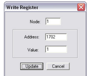
Figure 10-13: Modbus - write register - resetting the default values
