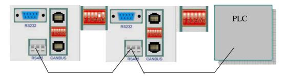
It is sometimes necessary to fix the potential of the RS485 + and – lines due to interference from other sources. This is done using two 1 k $\Omega$  resistors. One is fixed between RS485 + and +5 VDC, the other is fixed between RS485 – and the reference of the +5 VDC supply. The reference of the +24 VDC supply must then be connected to terminal 1 of the RS485 plug on each and every module.
