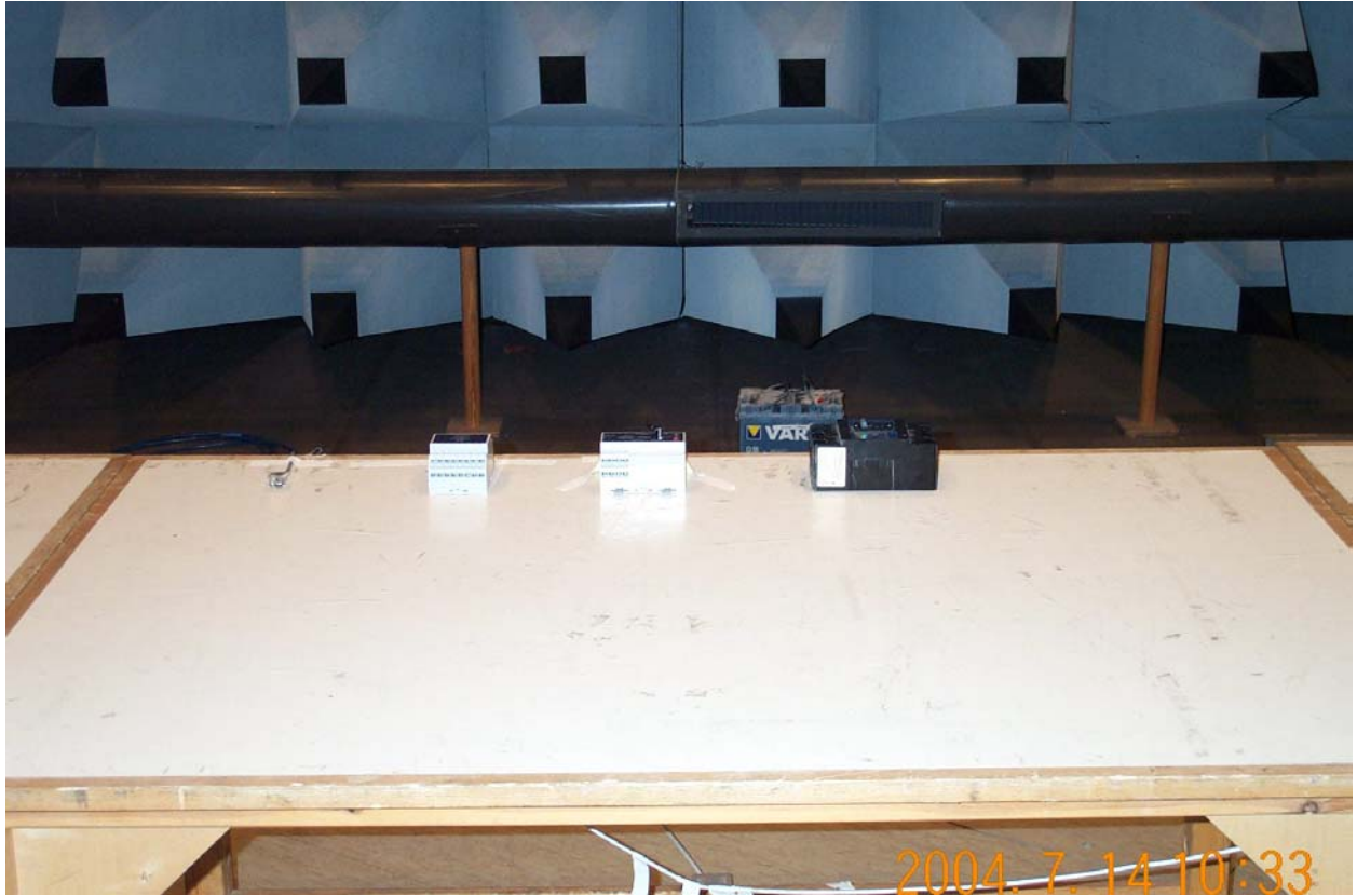
Photo A2.3 Radiated emission.
