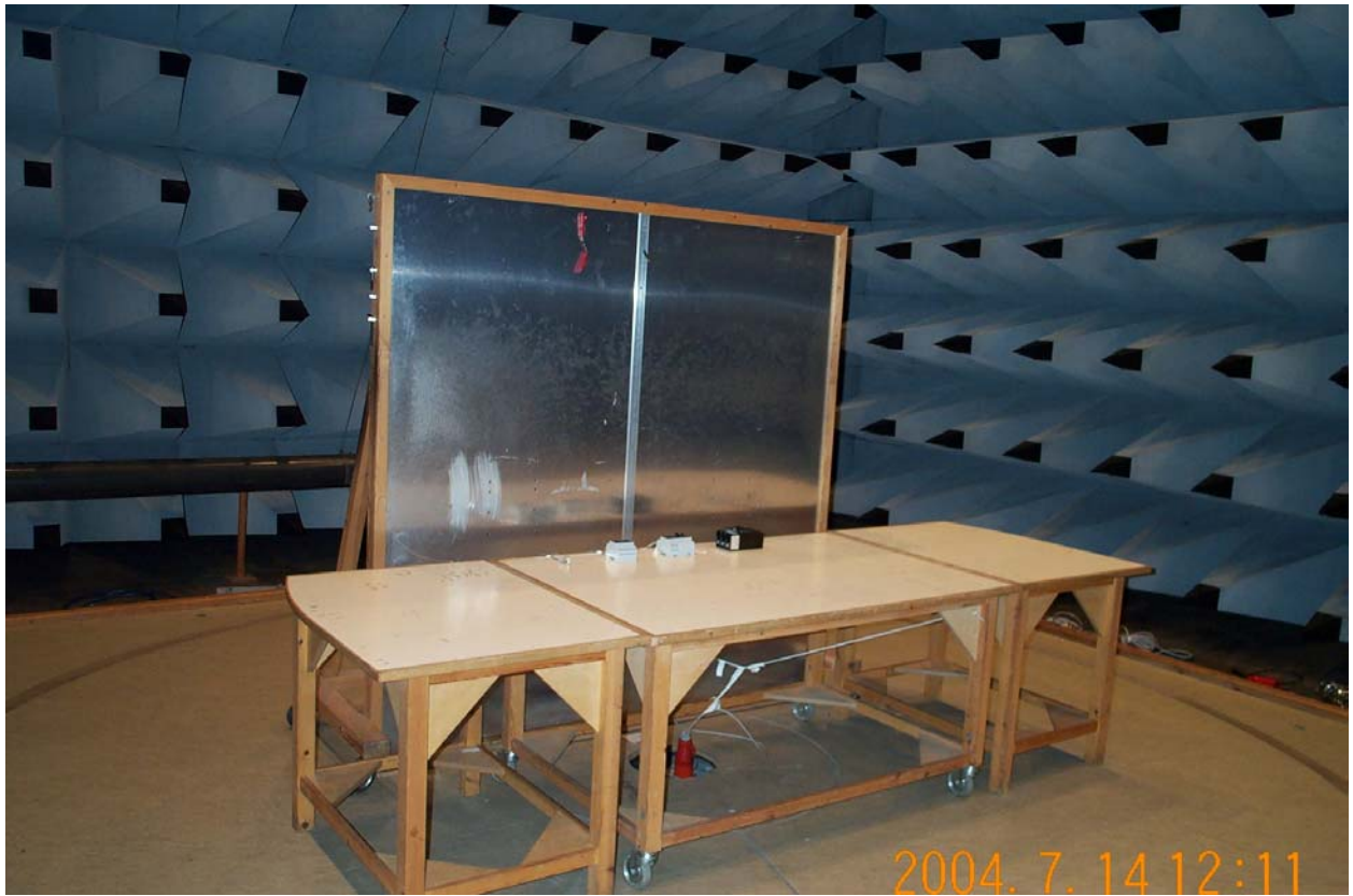
Photo A2.1 AC mains conducted emission.
