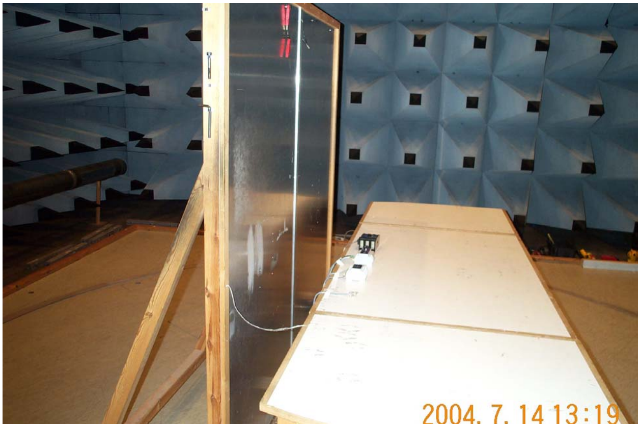
Photo A2.2 AC mains conducted emission.
