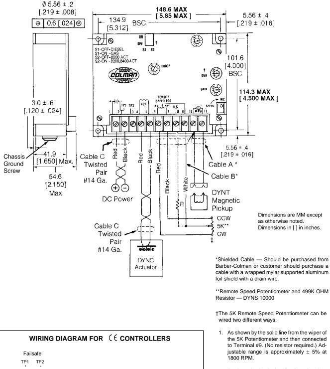
2. As shown by the dashed line from the wiper of the 5K Potentiometer through Resistor R and then connected to Terminal #8. Reducing the value of R increases the remote adjustable speed range.
